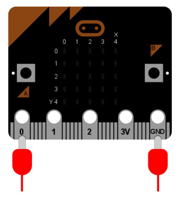
The wire from pin 0 should be attached to the positive connector on the speaker and the wire from GND to the negative connector.
