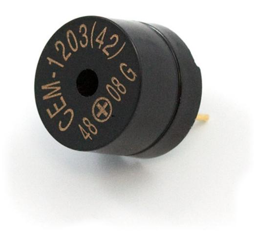
These small devices play a high-pitched bleep when connected to a circuit. To attach one to your BBC micro:bit you should attach crocodile clips to pin 0 and GND (as shown below).
