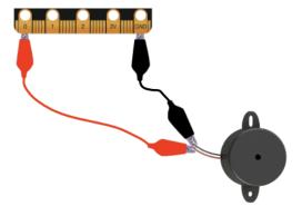
The wire from pin 0 should be attached to the positive connector on the buzzer and the wire from GND to the negative connector.
