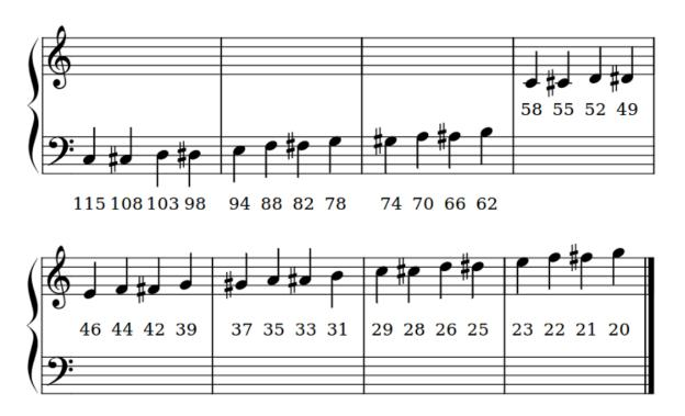
Annotations work by pre-pending a hash (#) sign and the pitch number in front of the phoneme. The pitch will remain the same until a new annotation is given. For example, make MicroPython sing a scale like this:
