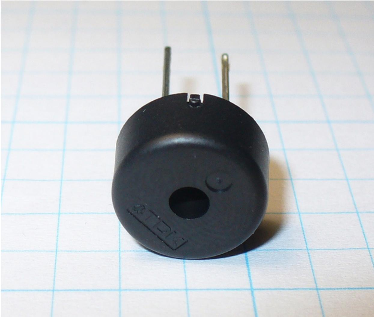
These small devices play a high-pitched bleep when connected to a circuit. To attach one to your BBC micro:bit you should attach crocodile clips to pin 0 and GND (as shown below).
