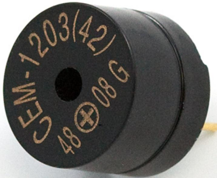
These small devices play a high-pitched bleep when connected to a circuit. To attach one to your BBC micro:bit you should attach crocodile clips to pin 0 and GND (as shown below).
