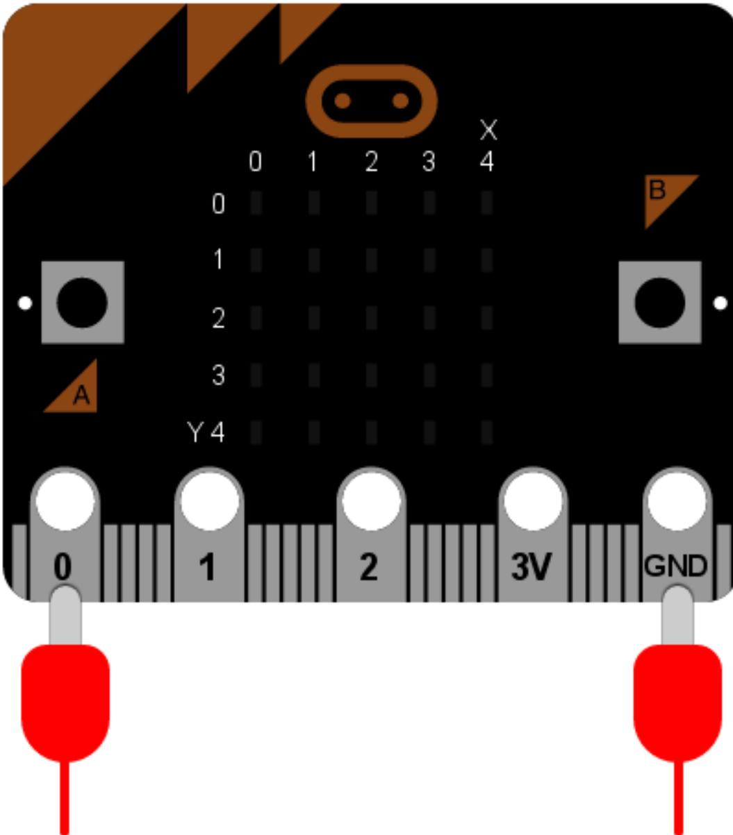
The wire from pin 0 should be attached to the positive connector on the speaker and the wire from GND to the negative connector.
